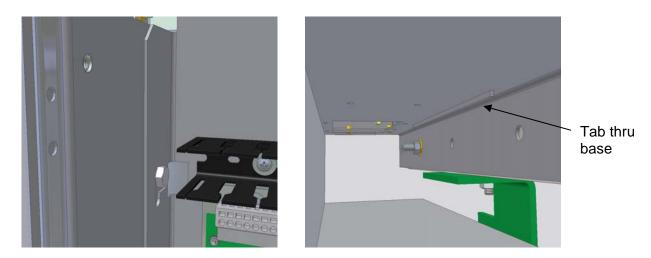
viii. Ensure that cabinet is square and level and that adjacent surfaces and edges are flush with each other and have minimal visible join lines. If not loosen Electrical Panel Bolts and Cabinet Frame bolts in area requiring adjustment and re-tighten.
